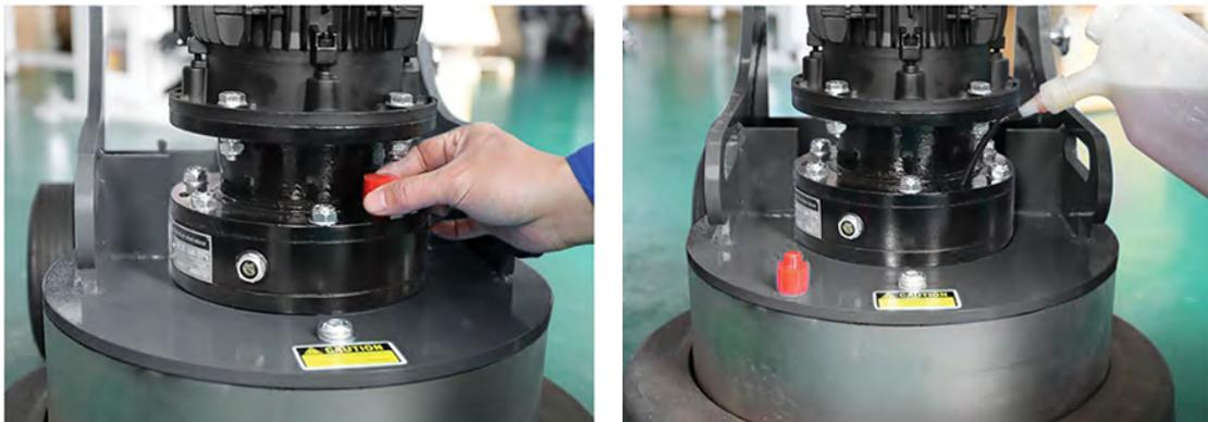
79. Every six months, clean the gearbox with a special detergent, and then replace the oil in the gearbox with new gear oil.
